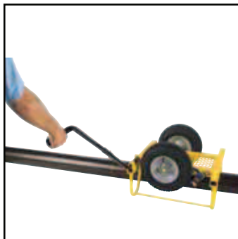
1 Use ratchet to secure Cricket to pipe
